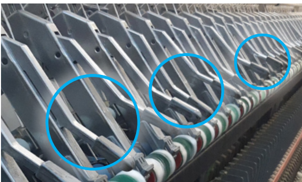
Before refurbishment – variation in load
