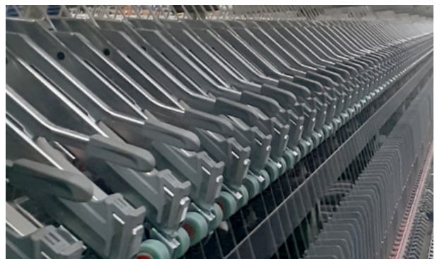
After refurbishment – uniform load
