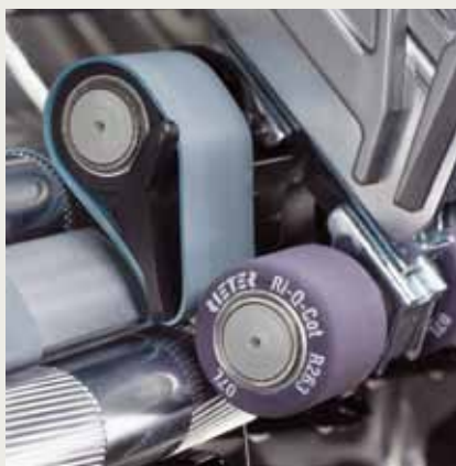
Ri-Q-Bridge in the drafting system
