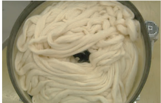
Fig. 1: Faulty first sliver coil
