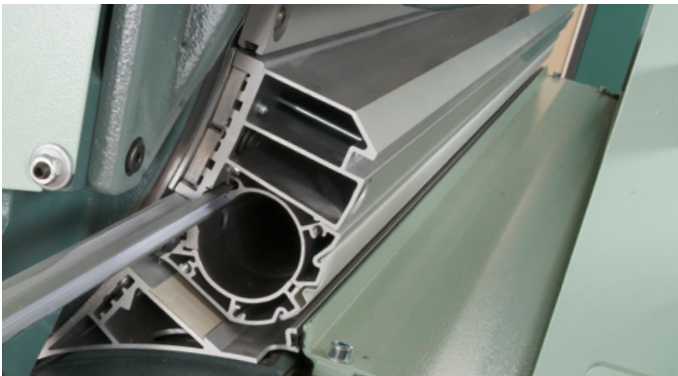
Inserts can be changed more quickly and easily for variable trash extraction.
