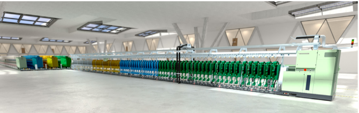
Up to four different lots can be processed on one Autoconer with Multilot
