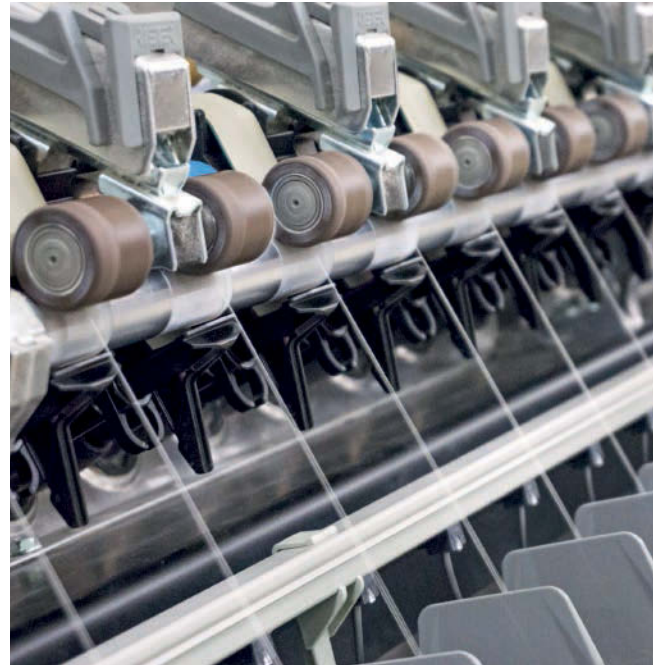
Fig. 2 The suction tube ECorized reduces the energy consumption of the ring spinning machine by approx. 10 %.
