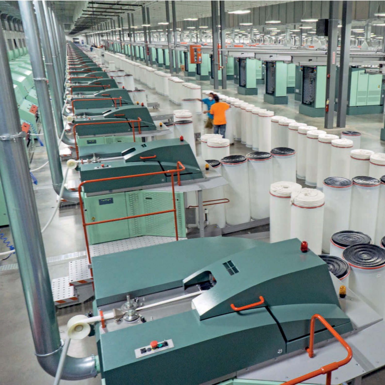
Fig. 2 C 70 Card with RSB-Module – Shorter processes and optimal sliver preparation for the rotor spinning machines.
