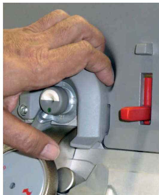
Fig. 3 The new S 66 spin box can be easily opened and saves the operator's time.
