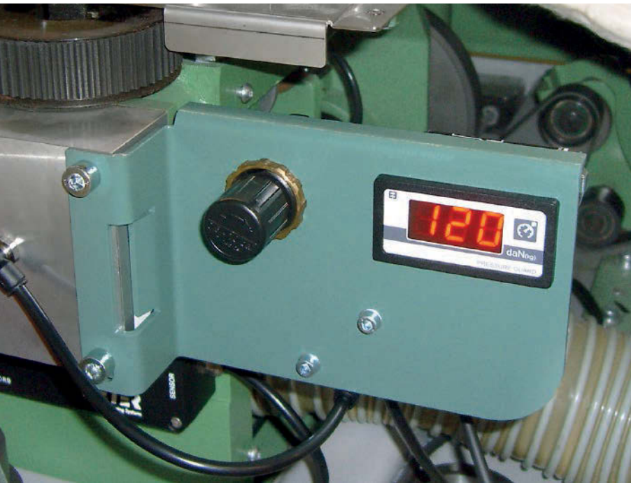
Fig. 1 On existing draw frames, the new compressed air monitor PRESSUREguard prevents uncontrolled and inferior sliver quality.
