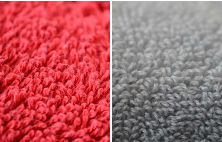
Fig. 3 Compared to the high-quality towel, the Rieter towel (right) made from Com4®jet yarn already performs extremely well visually.
