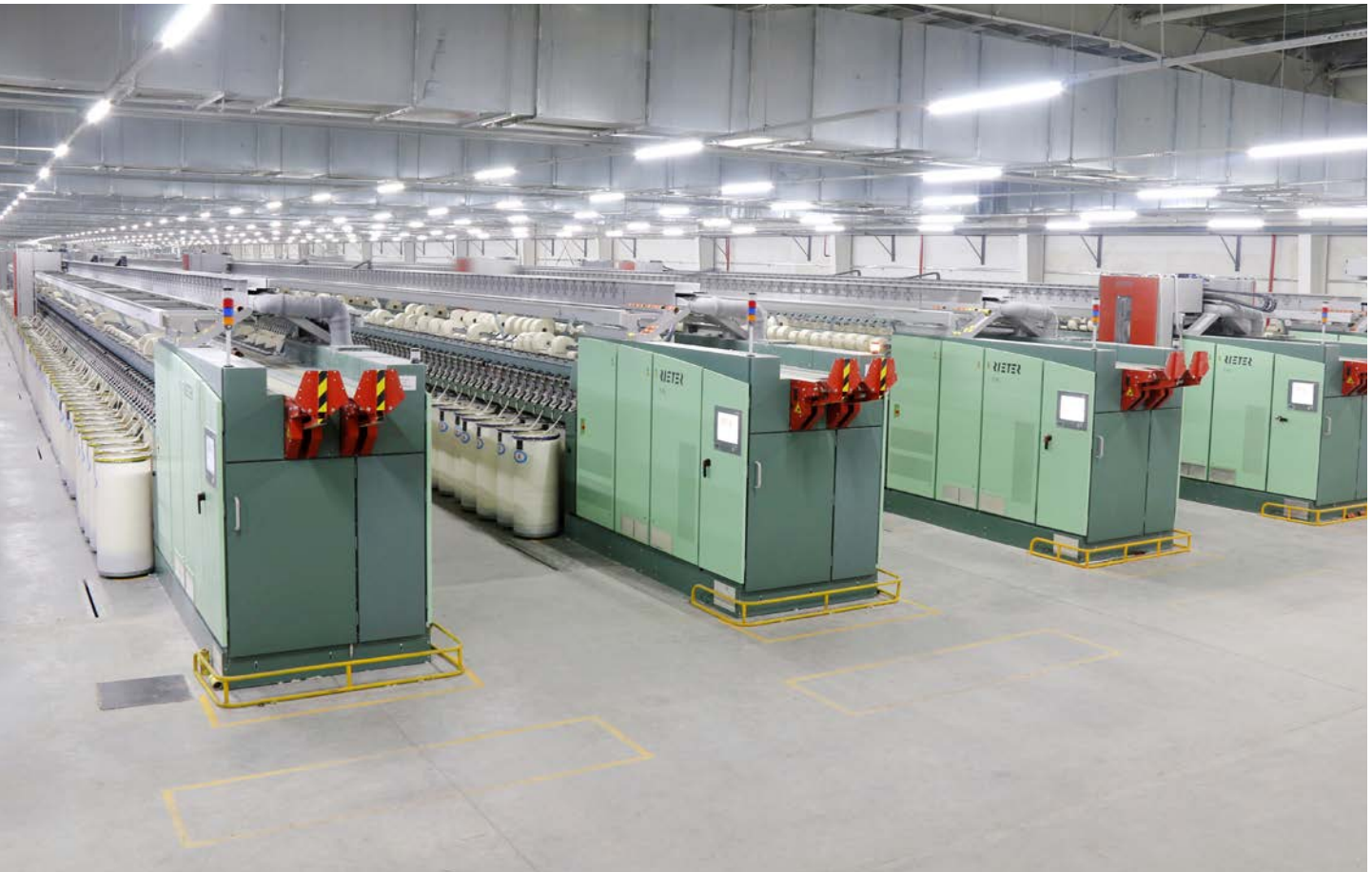
Fig. 1: R 66 Rieter rotor spinning machines at Xinjiang Kangruixin Textile Co. Ltd.: guarantees for soft knitting yarns and low production costs
