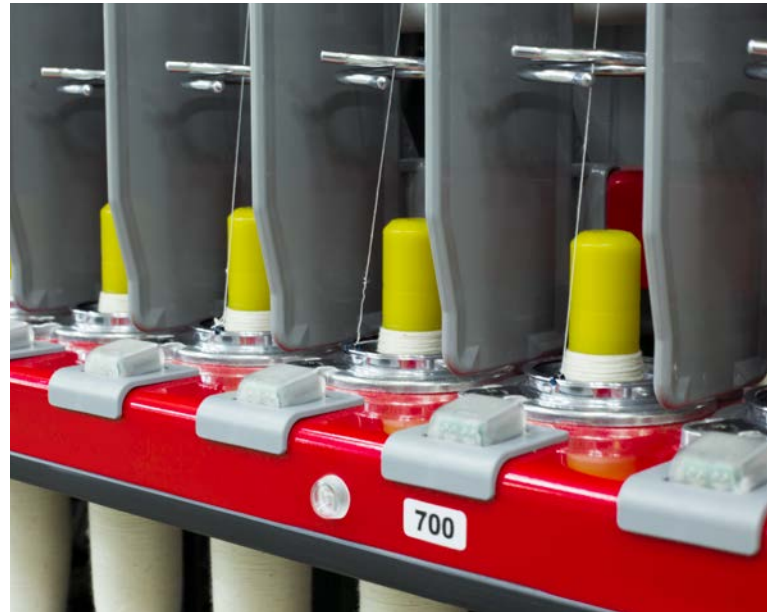
Fig. 2: The premium version of the individual spindle monitoring (ISM) is incorporated into the models G 38 and K 48. This reduces personnel requirements.
