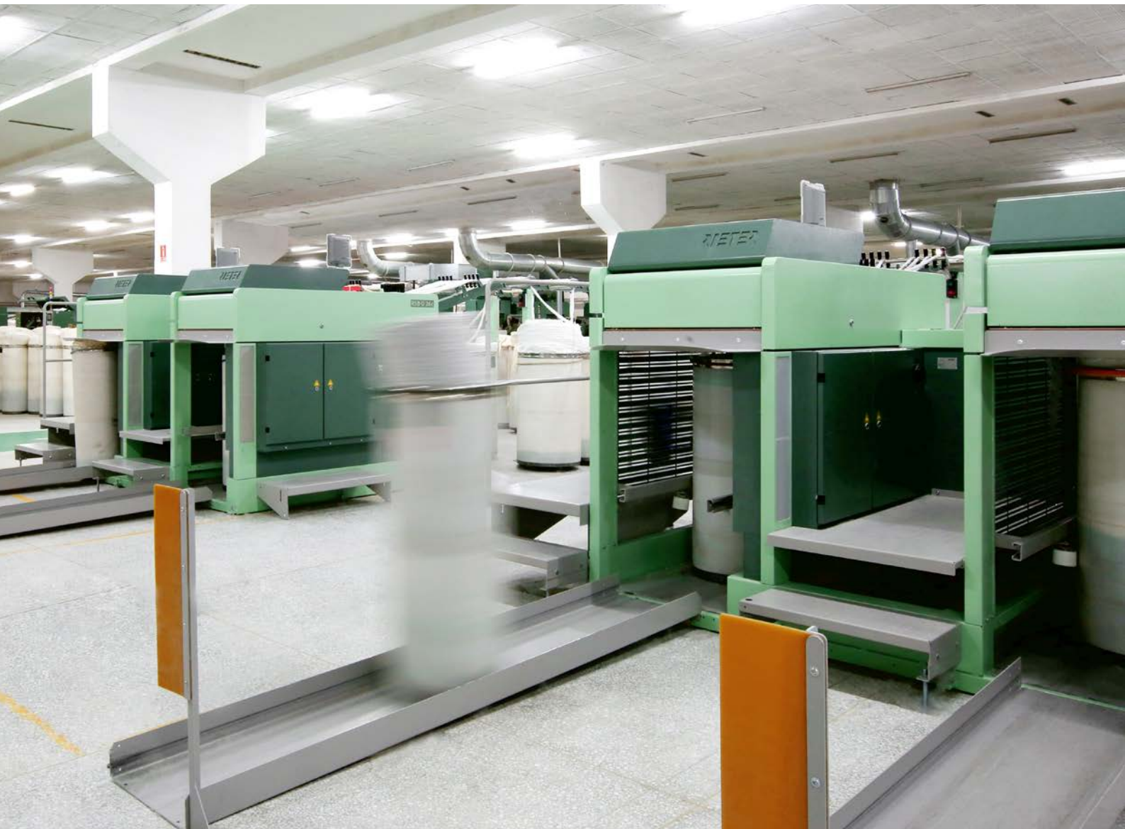
The new double-head autoleveler draw frame RSB-D 26 impresses with best sliver quality at highest productivity.
