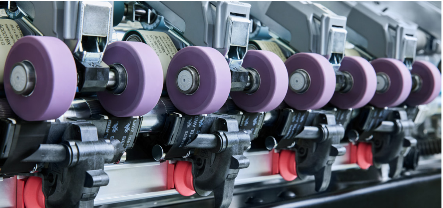
Fig. 1: COMPACTapron achieves higher tenacity values with an additional 0.5 to 1 cN/tex.
