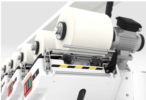
Counter-rotating blade system: the heart of the NEO-BD's yarn-friendly winding technology, enabling high speeds with minimal yarn stress
