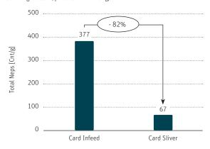
The sliver produced by the card C 80 is of the highest quality. The number of neps is reduced by 82% during the carding process.
