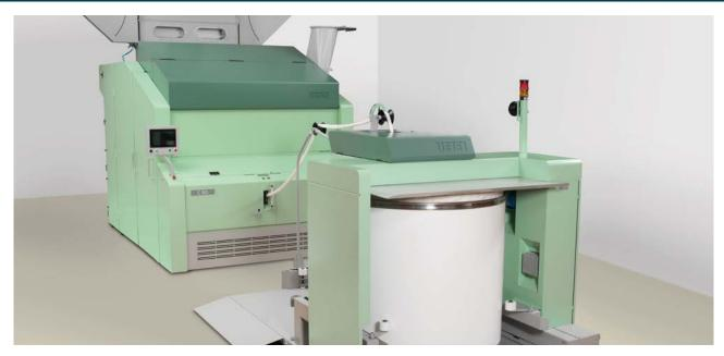
The high-performance card C 80 has been presented at ITMA 2019 for the first time and has since impressed numerous customers with its outstanding productivity. The performance of the C 80 during the last months at a customer has shown great results: The production level is higher by 67% in comparison to the C 70 for rotor fine yarn counts. The quality of the yarn and the production efficiency of the Rieter open-end machine is the same or even better.
