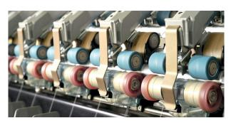
The G 37 with COMPACTdrum is hard to beat in terms of flexibility. Parameters such as yarn twist or twist direction can quickly be adjusted on the machine display. The compacting device COMPACTdrum can easily be plugged in or out and, as a result, enables the customer to switch between ring and compact yarn. The machine processes almost any type of fiber and can be easily and quickly adjusted to almost any raw material.
