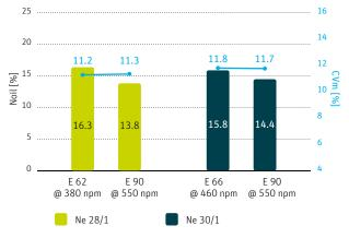
Consistent CV-values at a lower noil level compared to E 62 and E 66
