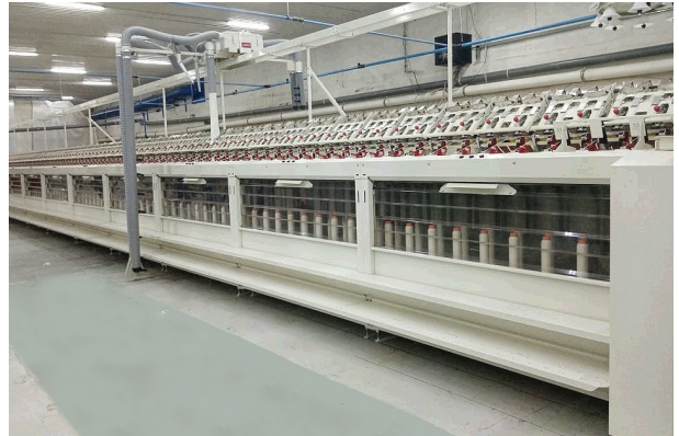
With up to 252 spinning positions, the F 40 is ideally suited for long ring spinning machines
