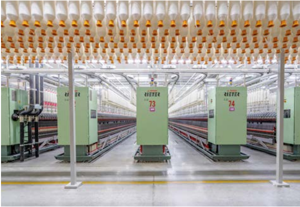
Ring Spinning Machine G 32 with compacting system EliTe®: maximum yield at low operating costs
