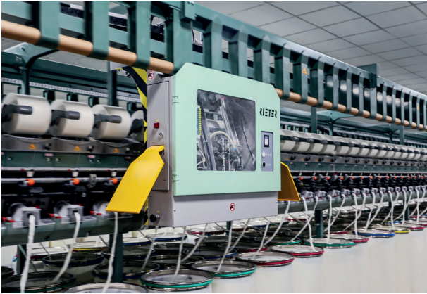
The Rieter R 37 rotor spinning machine with ROBODoff – maximum efficiency, consistent yarn quality, and enhanced competitiveness for Nuogao Fiber.
