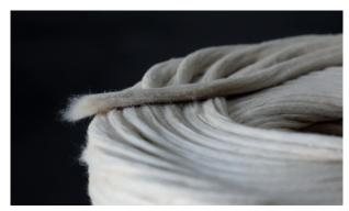
CLEANtube - the option for intelligent control of the coiler speed - avoids that trash particles and short fibers (called "mouse") accumulate on the top sliver layer.
