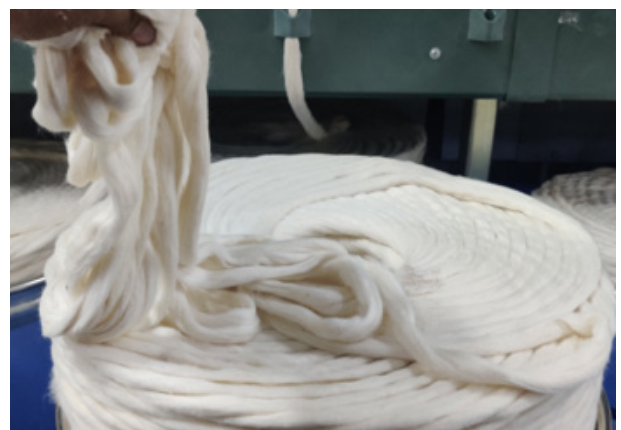
Fig. 2: Removing the mouse generates soft waste of about half a sliver layer
