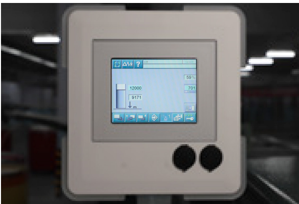
Fig. 4: Draw frame RSB-D 50 running speed at 701 m/min for spinning special fibers
