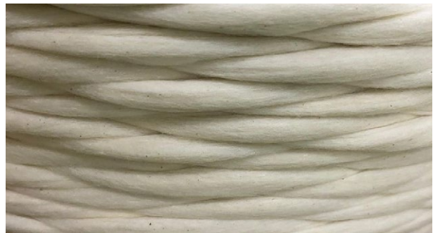
Sliver produced with the C 75 and RSB-Module 50
