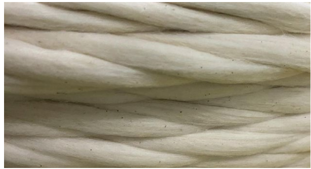
Sliver produced with the competitor's card and integrated draw frame
