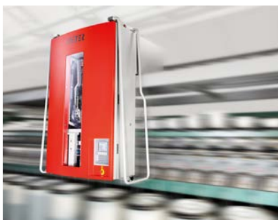
Additional robot on fully-automatic rotor spinning machine
