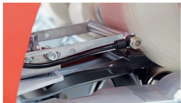
The Smartjet power nozzle – in the doffer – increases the success rate of upper yarn searching even further.
