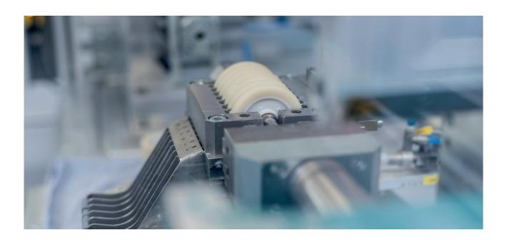
With increasing texturing speed and finer filaments, the negative effect becomes more serious. PU discs are softer than the yarn, handle the yarn with care during twist insertion. The best yarn quality is based on careful selection of PU material, disc geometry and surface structure. Numerous tests with strict limits keep the texturing performance of Temco discs within narrow limits.
