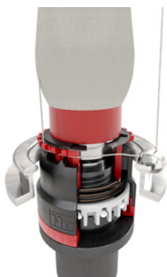
Cop is finished, Back-winding, Yarn inserted.
