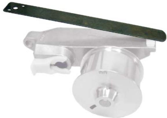
The new flat spring of the Performance Kit reduces the load to the contact roller suspension and thereby achieves energy savings up to 18% to 20% (depending on the rotor speed – see light-green line in Fig. 2).
