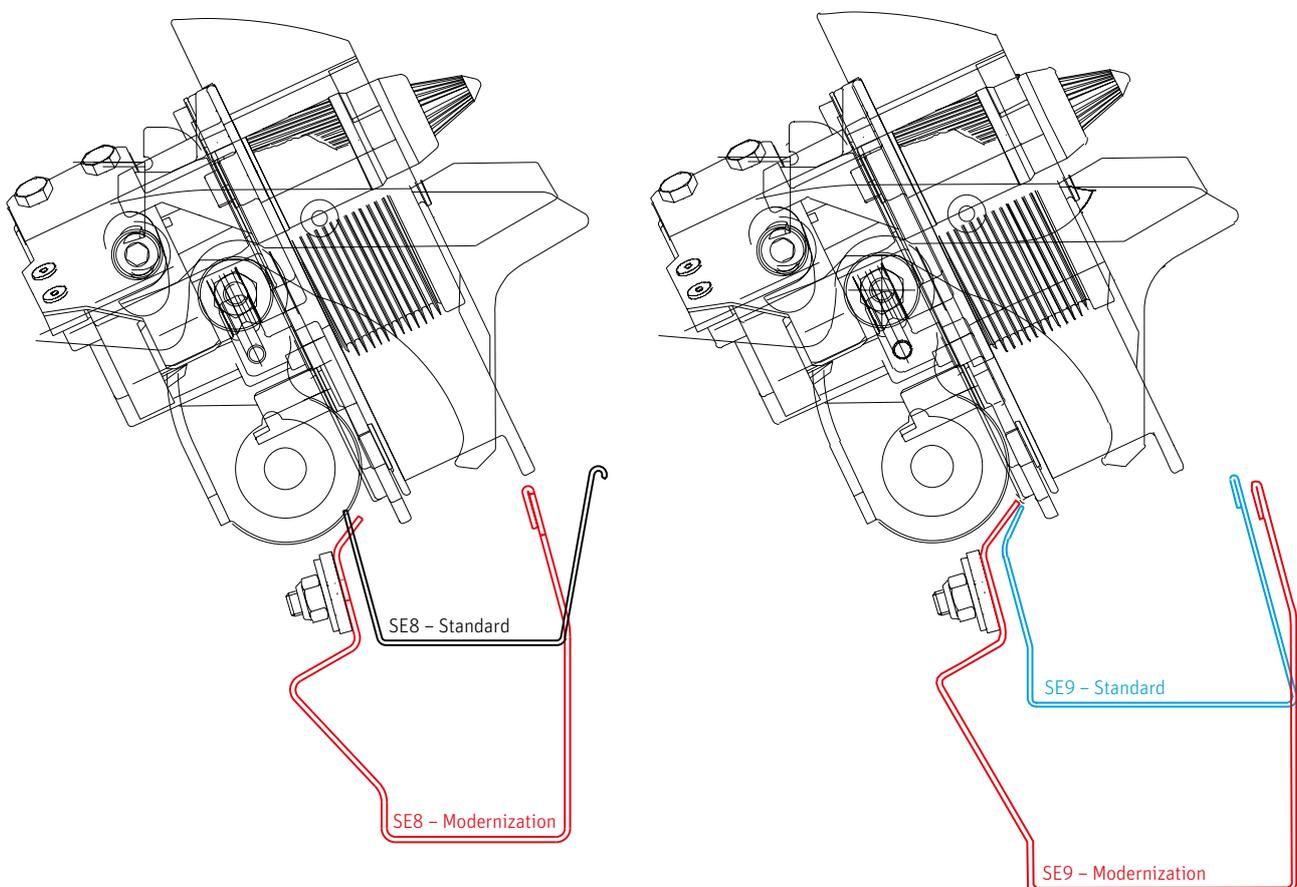
In fact, the only component to be replaced is the trash channel. The complete drive system of the trash conveyor belts is reused as well as the conveyor belts themselves. Consequently maintenance, settings and spare parts of the trash removal system remain the same. This is very comfortable for your spare parts stock and the maintenance personnel.
