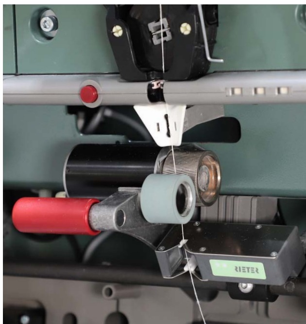
Delivery with single drive of AMIspin-Pro (above) or with delivery shaft of AMIspin (right)
