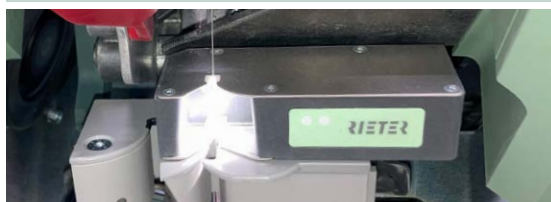
Stepless clearing curve and wide measurement area of the yarn clearer Q 30
