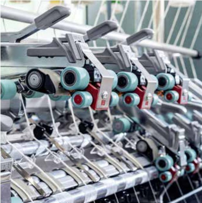
Fig. 6: Transmission of the traverse motion to the Compactor
