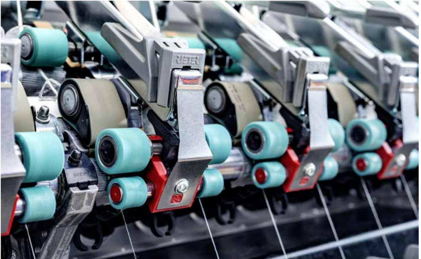
Fig. 3: COMPACTeasy on Rieter P3-1 top weighting arm
