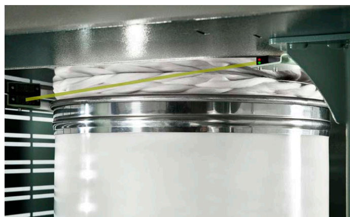
Light barrier for controlled sliver coiling
