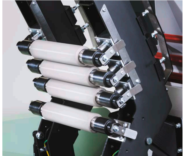
Top rollers with optimized load distribution
