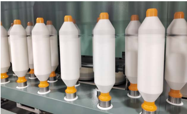
Precise bobbin build-up for high-quality roving
