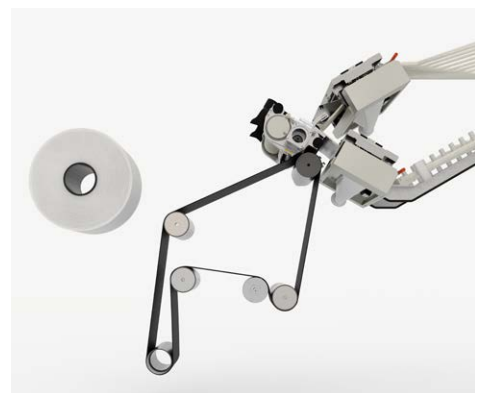
3. Ejecting the full lap through belt tension
