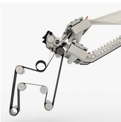
1. Putting the empty tube into the belt
