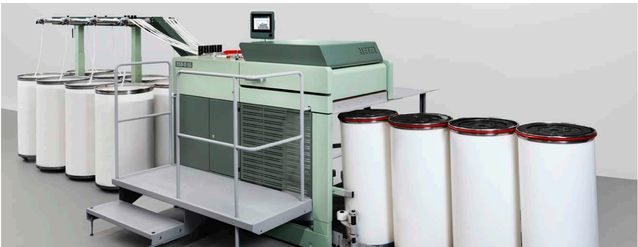
Rieter's Autoleveller Draw Frame RSB-D 55 for stable operation with high quality and productivity
