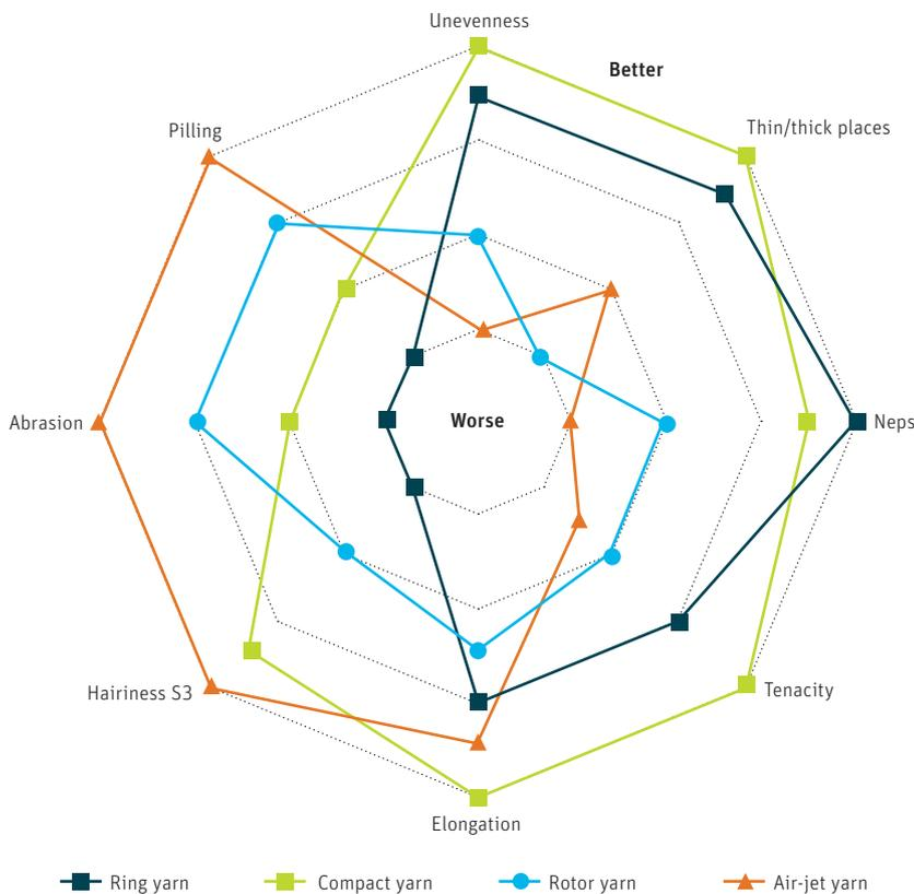
Fig. 15: Depending on the spinning process, the yarns have various properties and are suitable for different applications.
