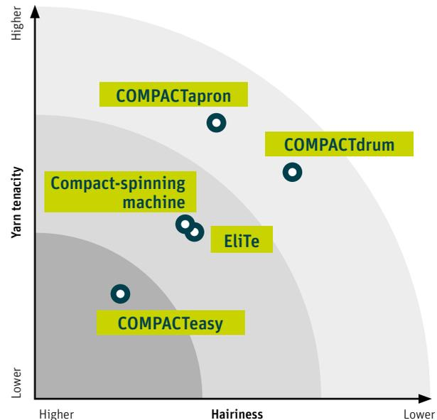
Fig. 2: Positioning of the three Rieter compacting devices in comparison to the compact-spinning system EliTe and the compact-spinning machine with pneumatic compacting.
