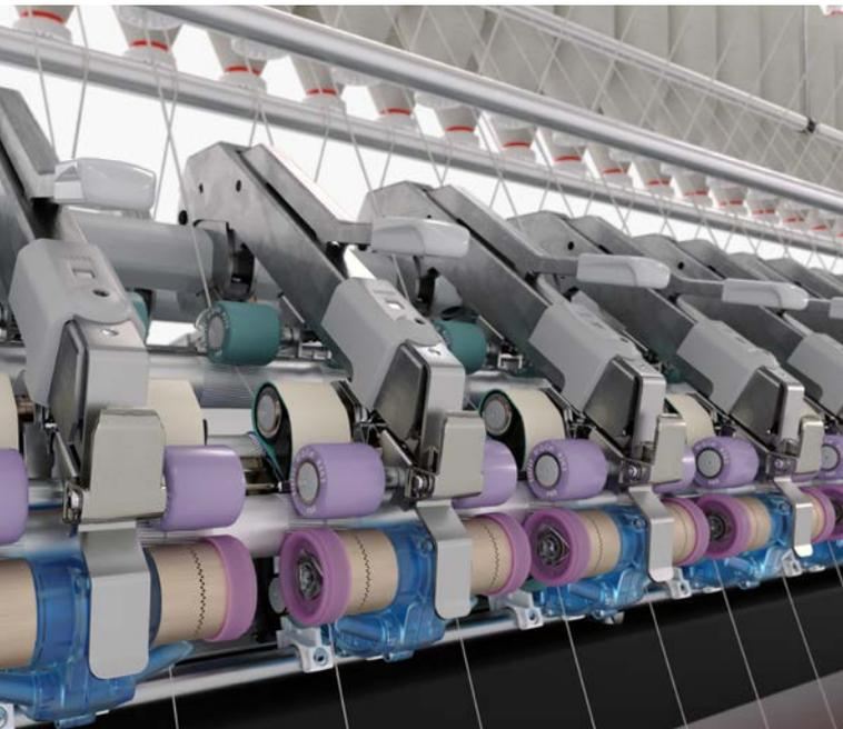
**Fig. 1:** Ring spinning machine G 38 with the fully electronic drafting system drive and compacting device COMPACTdrum for simple switching between ring and compact yarn
