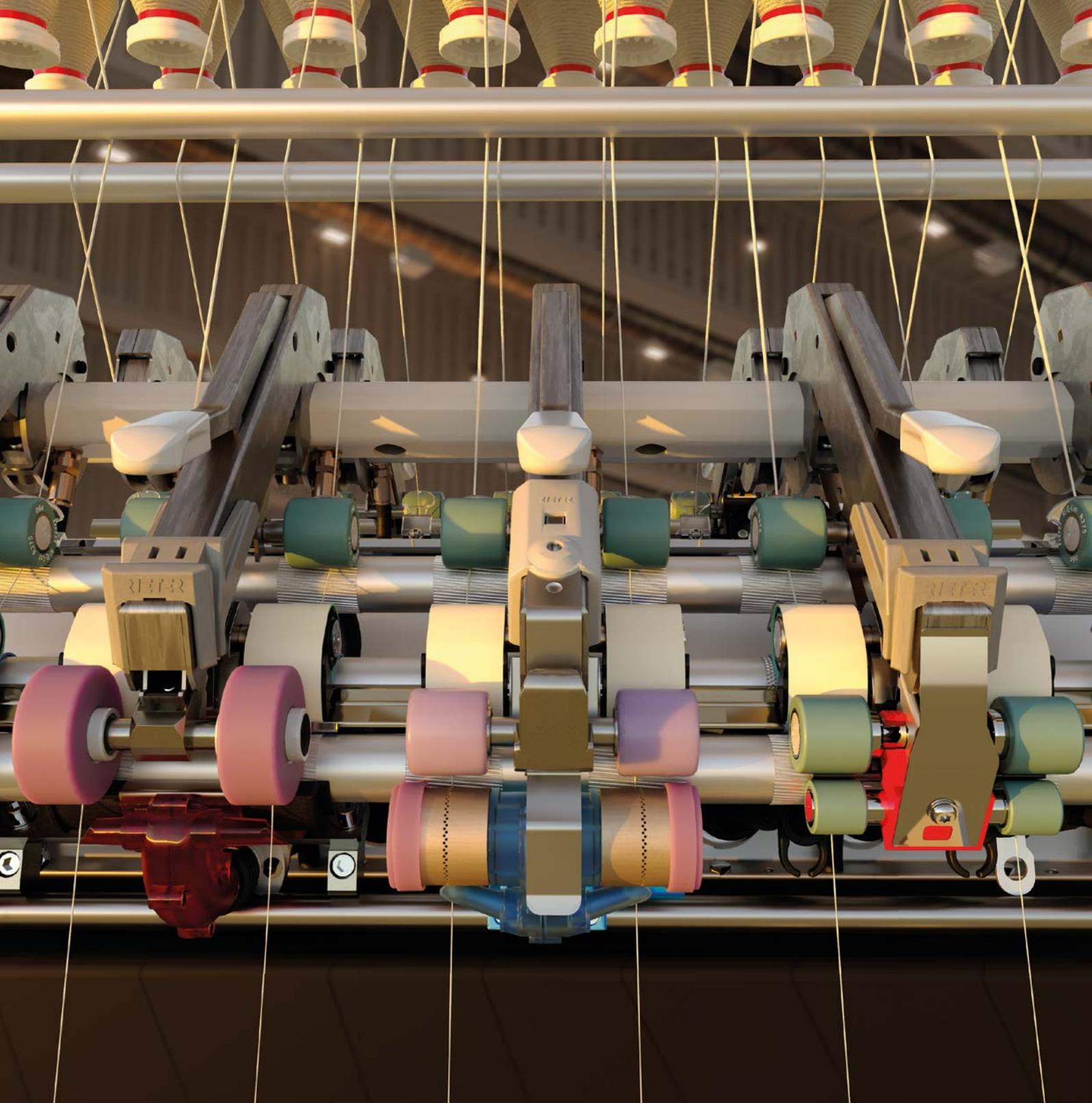
New compacting possibilities: spinning ring yarns and compact yarns using the same machine
