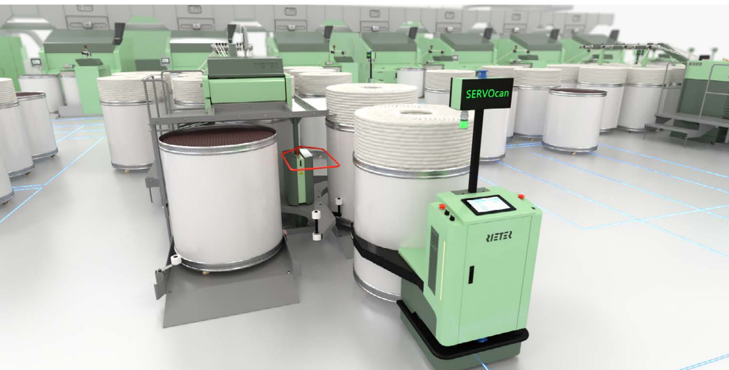
Fig. 1: Step-by-step to a fully automated Rieter spinning mill with only three operators for every 10 000 spindles and 1.9 tons of yarn per shift (based on: 100% combed cotton, yarn count Ne 30, weaving yarn).
