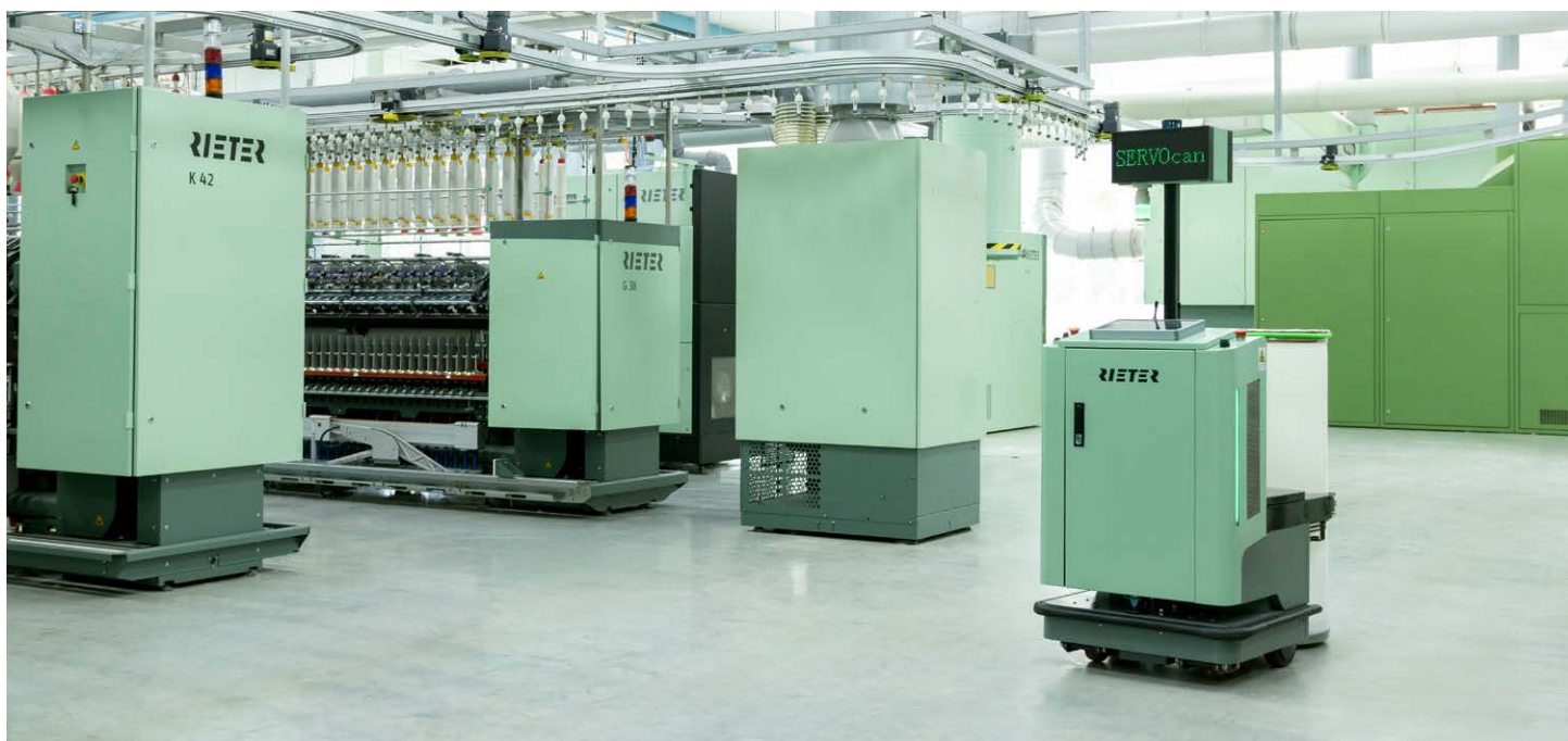
Fig. 2: Automatic can transport takes over monotonous and physically demanding tasks.
