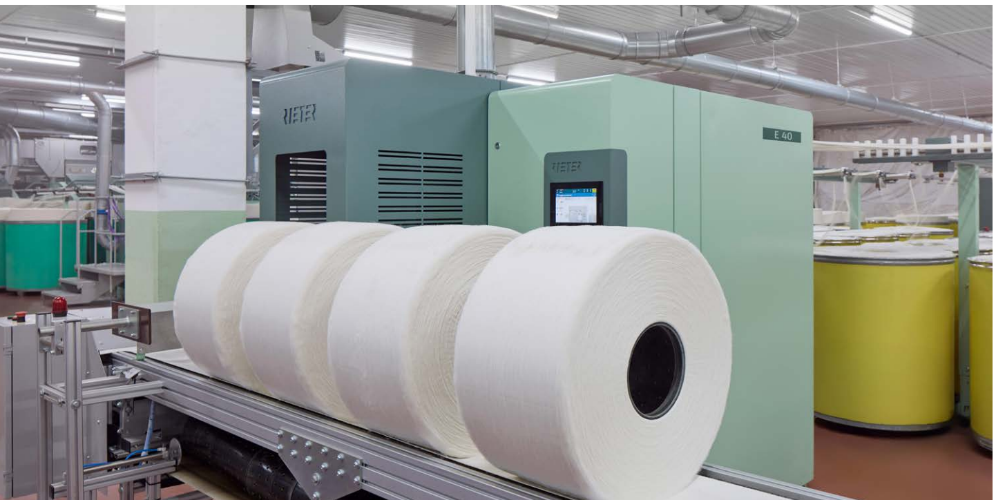
Fig. 1: The new combing preparation machine OMEGAlap E 40 scores with fast lap changes and easy maintenance.
