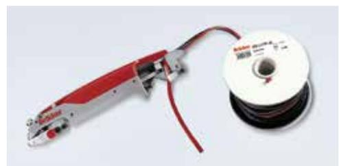
The travellers are lined up on a profile strap (up to 10,000 pcs per spool) The STRAP System is applied for SU travellers for ORBIT spinning rings and for C-shaped travellers with „fr“ profile.
