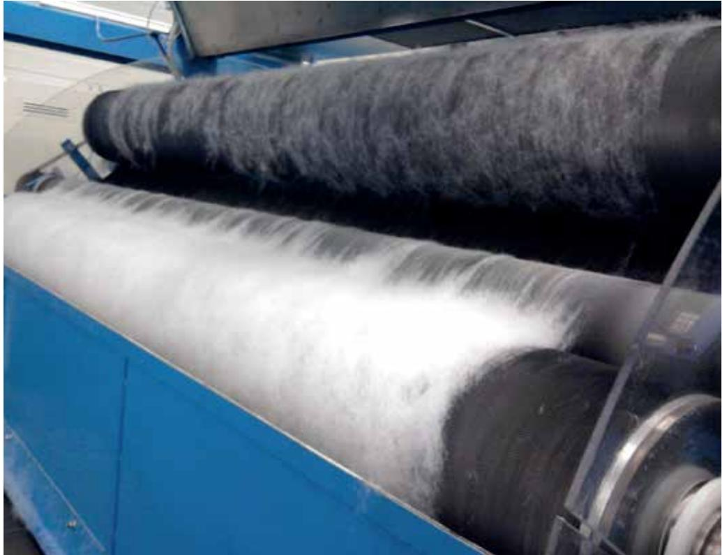
Fig. 7 Adhesion of fibres with Hipro. Bottom worker roller clothed with Hipro, top worker roller clothed with standard metallic wire.
