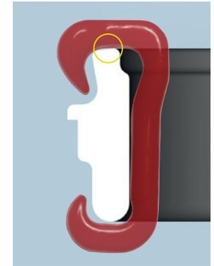
Excessive wear on head – tension is too low
