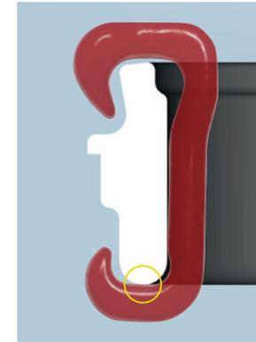
Excessive wear on foot – tension is too high
