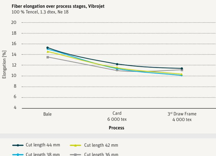
Fig. 8 Fiber elongation over the process stages
