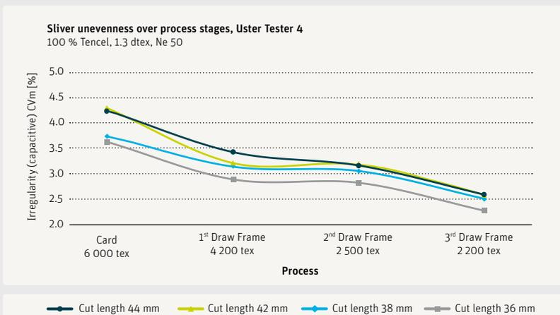
Fig. 9c Sliver irregularity over the process stages
