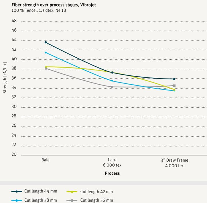
Fig. 7 Fiber strength over the process stages
