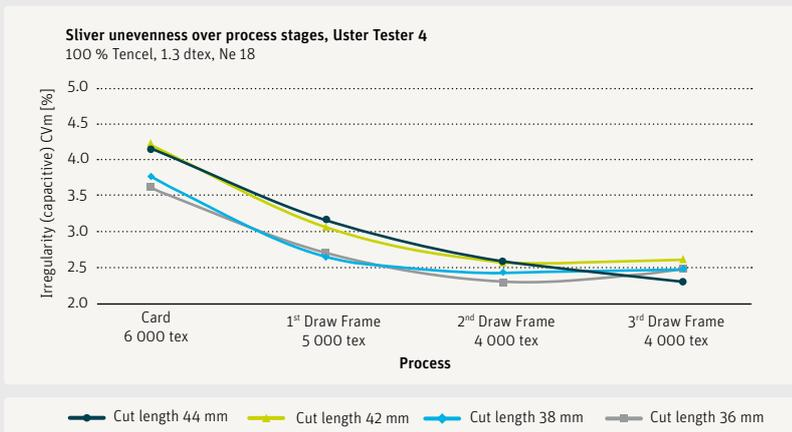
Fig. 9a Sliver irregularity over the process stages
