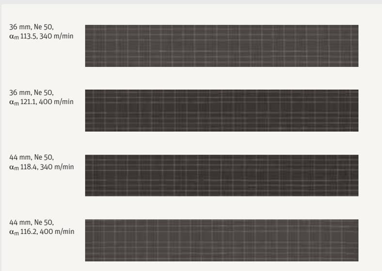
**Fig. 44** Fiber shifting
