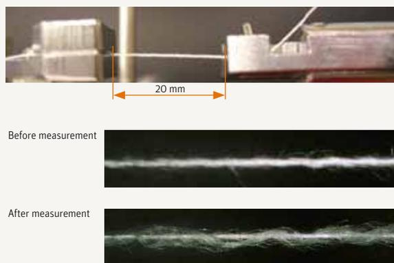
Fig. 33 Microscopic measuring method
