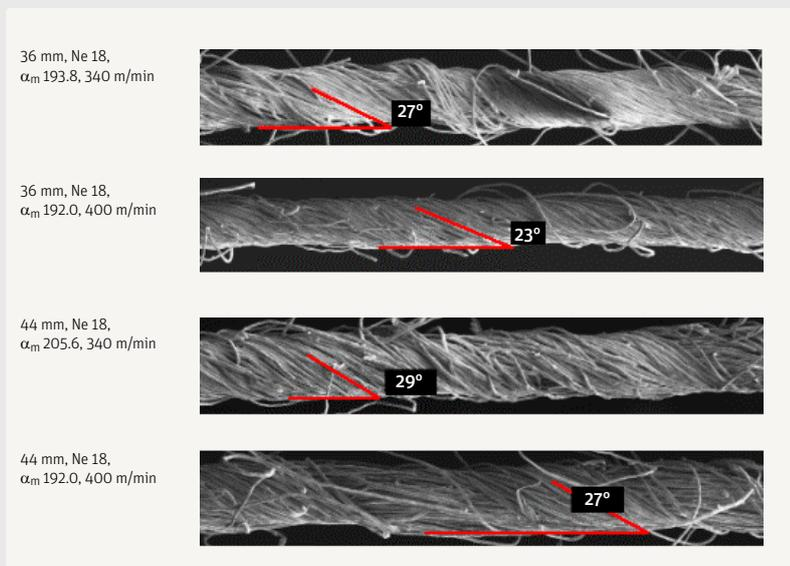
Fig. 37 Yarn twist angle
