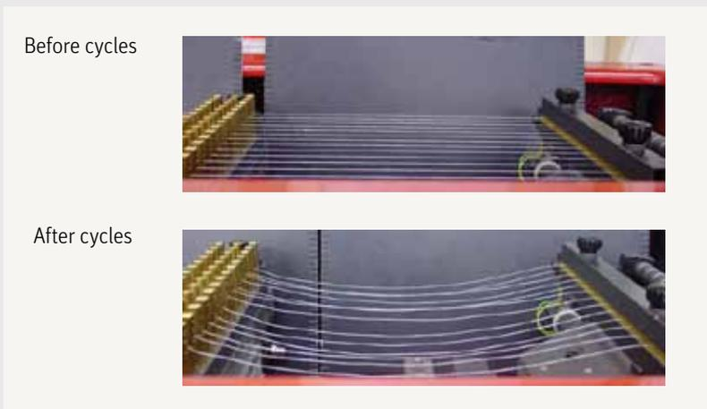
Fig 41 Plastic deformation of the yarn
