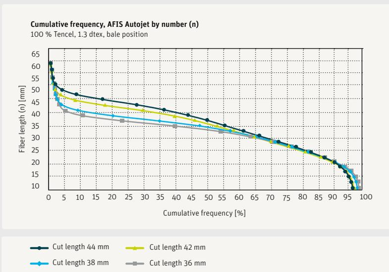
Fig. 10 Staple diagram of the different cut staples
