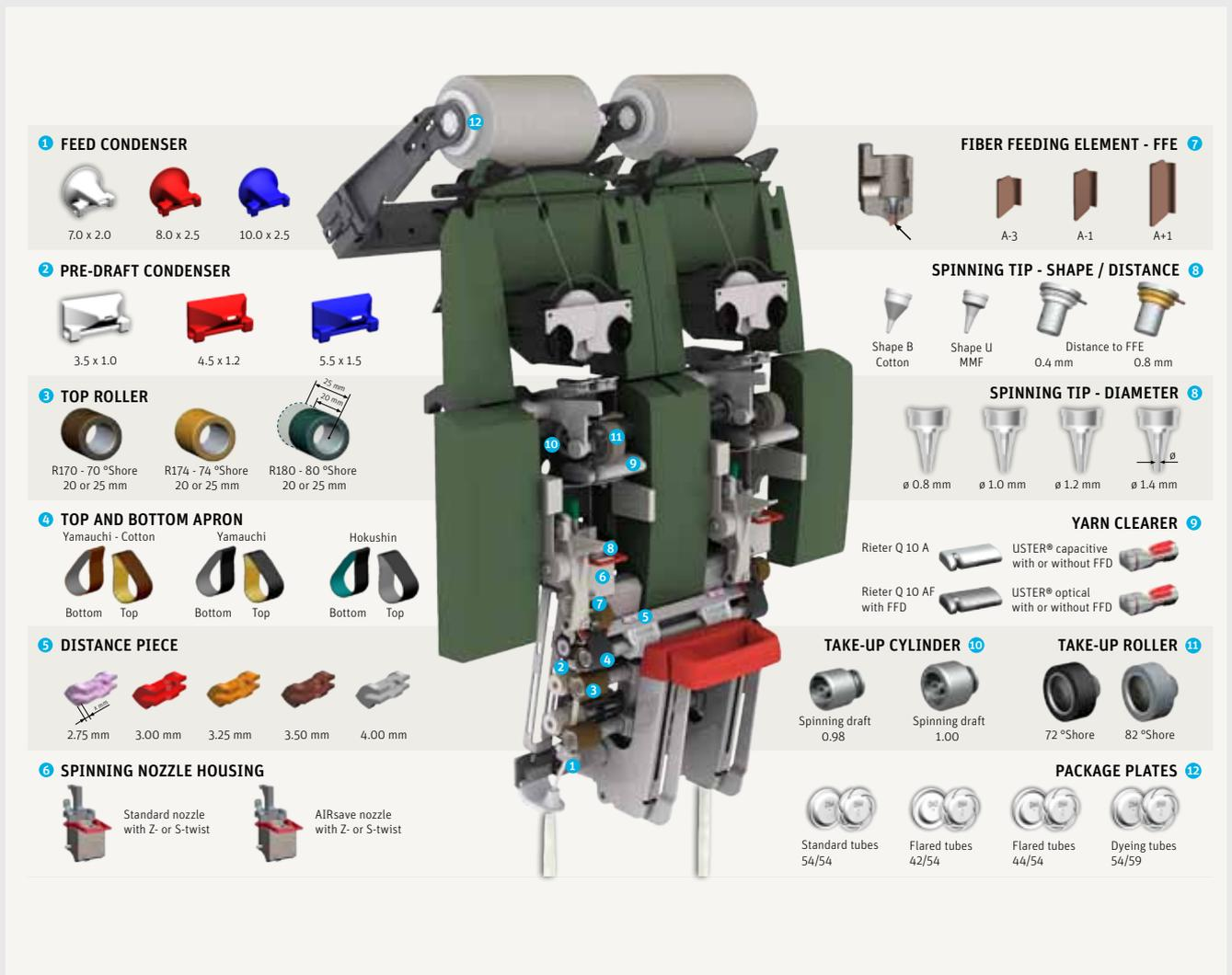
Fig. 47 Technology components
