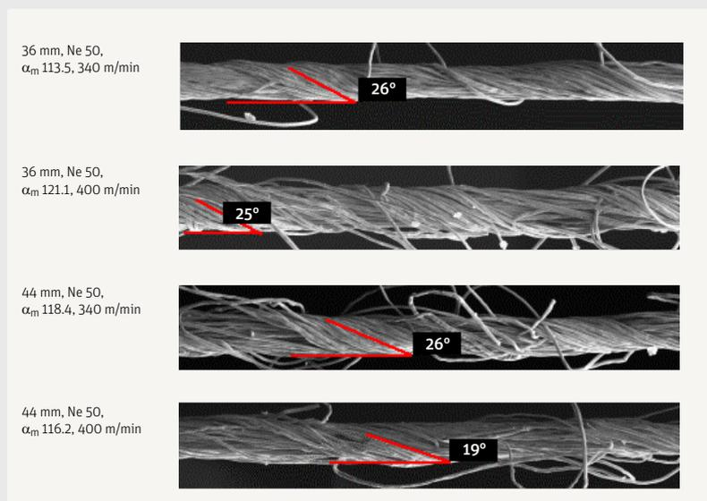
Fig. 38 Yarn twist angle
