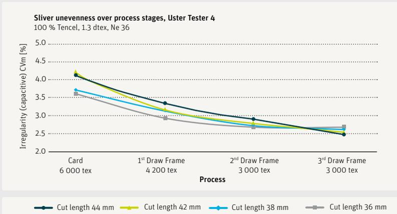
Fig. 9b Sliver irregularity over the process stages
