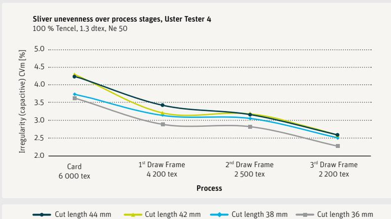
Fig. 9c Sliver irregularity over the process stages
