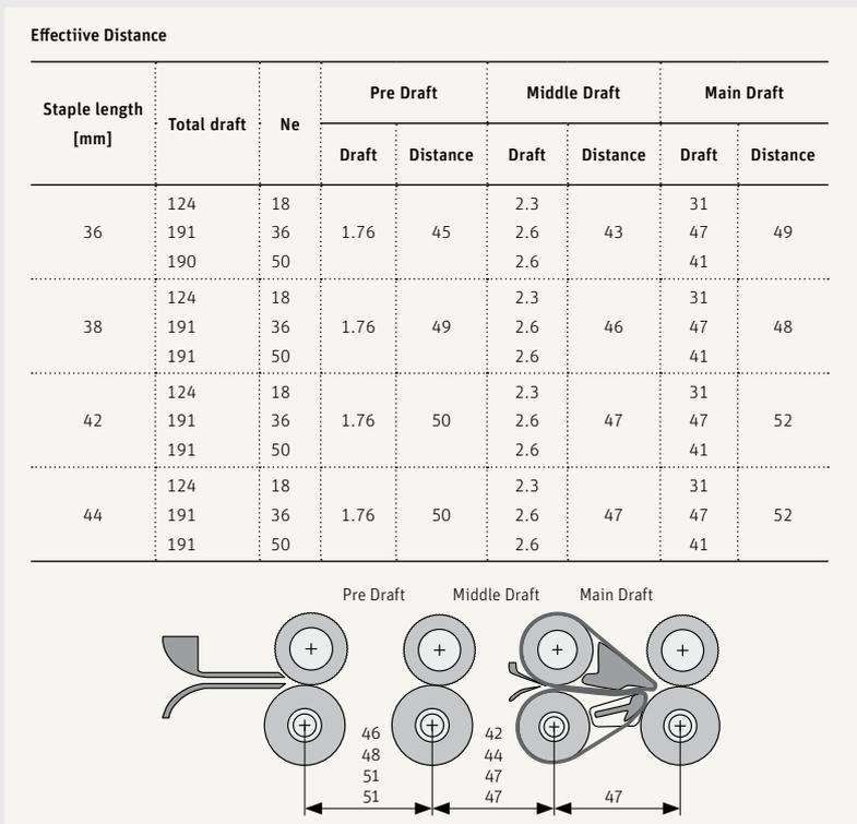
Fig. 11 Draft settings (break, intermediate and main draft)
