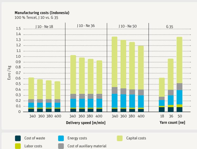
Fig. 46 Yarn manufacturing costs: air-jet-spun yarn vs. ring-spun yarn
