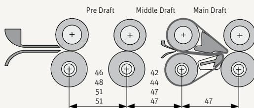
Fig. 11 Draft settings (break, intermediate and main draft)
