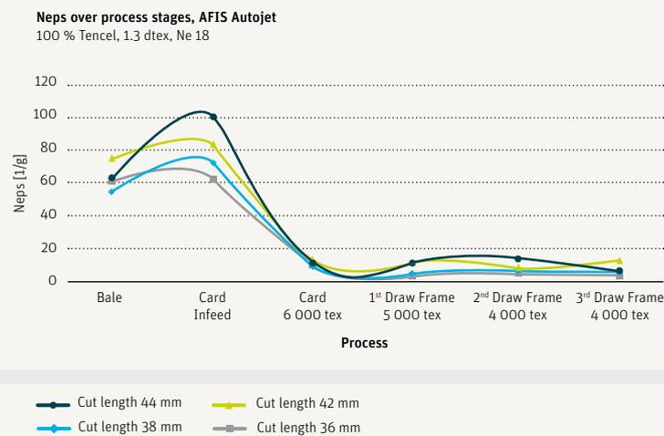
Fig. 6 Number of neps over the process stages
