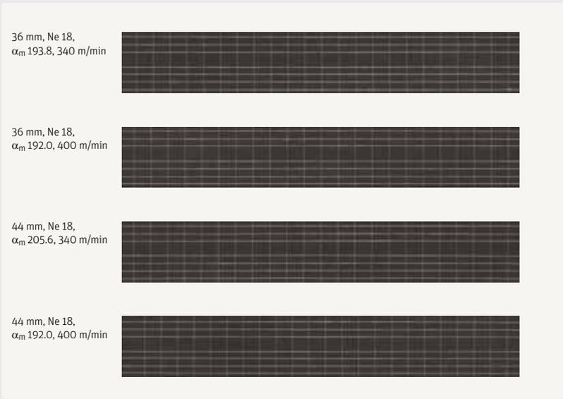
Fig. 43 Fiber shifting
