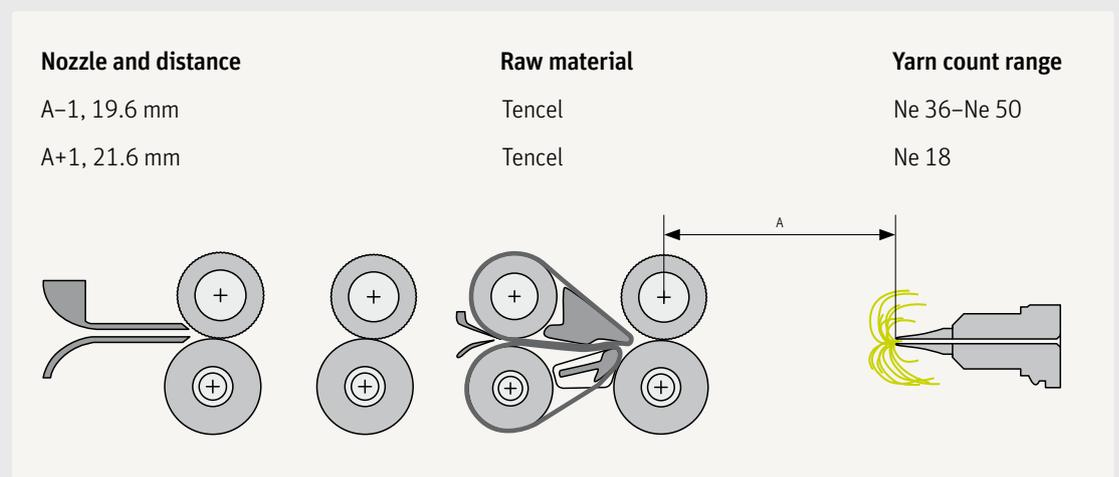
Fig. 12 Spinning nozzle spacing
